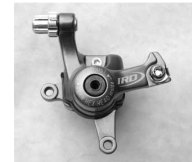
FIG. 2: REAR DISC BRAKE DOES NOT NEED THE INT'L STANDARD ADAPTOR. IT BOLTS RIGHT ONTO FRAME
