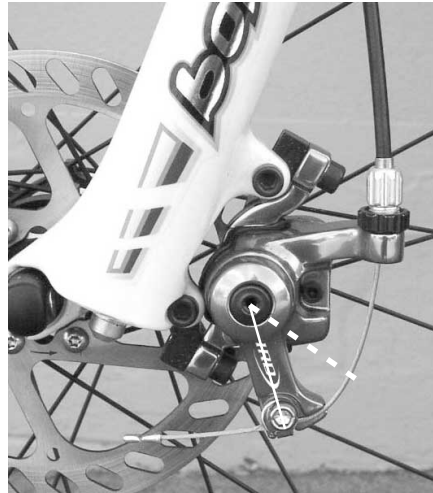
FIG. 5: Brake installed on frame using IS adaptor. Note how cable is installed. When brake is actuated, the arm is not supposed to go beyond dotted line (about 30° of motion) If it does, your pads have worn and you need to move pads closer to the rotor.
